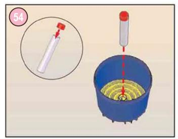
Place the cap on the collector pipe and insert it into the hole in the middle of the collector plate. Pour the sand filter medium carefully into the tank, use your hand to spread it out evenly.
