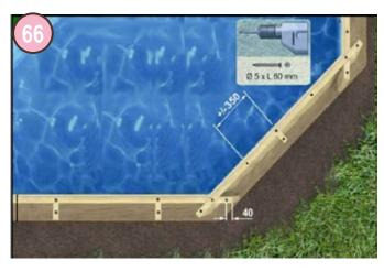
Attach the 7 coping planks of the same length. Be careful to drive the screws into the centre of the wooden walls to avoid damaging them. (screws from bag T or Q)
