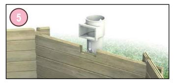
At this point, fit the skimmer or autonomous filtration unit into the bottom skimmer slat (type D).
