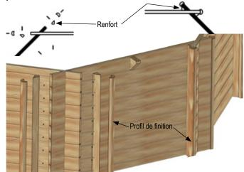
To attach the brace from the outside: locate the screws 100mm from the corner. Use one screw per slat.
