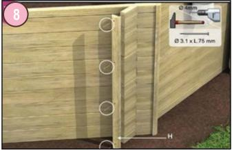
Mount a decorative profile (type H) on the end of each wall using nails (3.1x75mm) inserted through evenly spaced holes pre-drilled along the axis of the profile.
