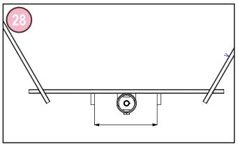
Mount 2 wooden brackets on the wall holding the skimmer, they should be positioned equidistant from the skimmer axis. The distance between the 2 brackets varies depending on the pool model, see the table below.
