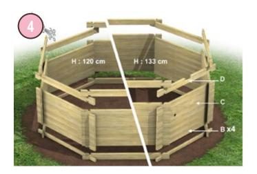
Fit together the remaining slats (type B) taking care to position the slat that will hold the return fitting (type C) and the machined slat (type D) correctly. The slat that will hold the return fitting should be positioned over 4 (type B) slats + 1 type A slat in the case of a skimmer and an autonomous filtration unit. The return fitting slat should be located just under the machined (type D) slat which should be in the last row of slats at this point in the assembly.
