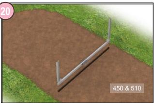
Once the cradles have been assembled, place them in the trenches and block them in position using wet compacted sand if necessary. During this operation, check that the cradles are level, straight, aligned and parallel. Fill the trenches using wet compacted sand.
