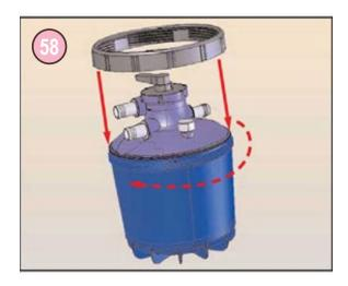
Put the lid ring into position to hold the lid on the tank.
