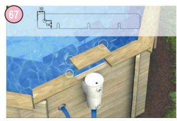
Before fastening the 3 parts of the coping over skimmer in position, pre-drill the central element and the two side elements at the points indicated above. Make sure that the holes (6mm) are drilled very precisely and that they are properly aligned. Insert the pivots (bag ref 27511070), then replace the coping elements..
