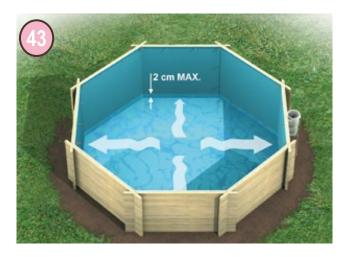
Once the liner has been hung and is correctly positioned, fill the pool with 2 cm of water. Push any creases towards the walls smoothing out the liner as much as possible. Take care to ensure that the floor is as smooth as possible. This operation will not be possible if the pool is empty or overfilled (contains more than 2 cm of water).
