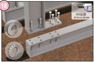
Lay the cradle components out beside the trench and fit them together (using the cradle kit).
