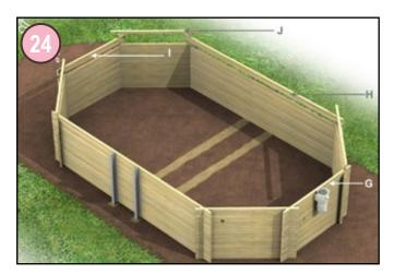
At this point, fit the skimmer into the machined slat (F). Slot the top skimmer slat (G) over slat F and continue around the pool, fitting 2 type H slats, 1 type I slat and 4 type J half-slats into position as shown.
