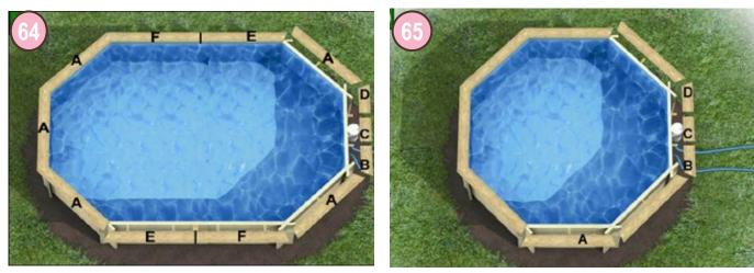
Note the distribution of the various modules constituting the coping on the drawing. Arrange them on the coping support brackets. Make sure that the elements are correctly and evenly positioned around the entire periphery of the pool. Adjust them if necessary and make sure that they remain in position until screwed in.
