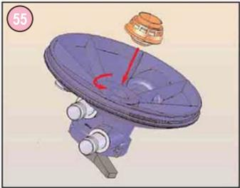
Insert the diffuser into the lid and rotate it anticlockwise to lock it in position.
