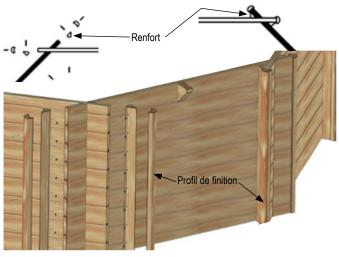
To attach the brace from the outside: locate the screws 100mm from the corner. Use one screw per slat.
