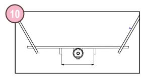
Mount 2 wooden brackets on the wall holding the skimmer, they should be positioned 75 cm apart and equidistant from the skimmer axis.
