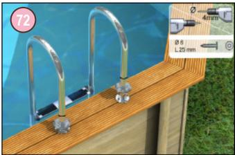
Position the ladder in the pool on the coping module of your choice (except the wall holding the skimmer and counter swim module), remember that it should be opposite the wooden ladder.
