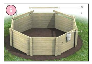
Fit the two slats at aither side of the filtration unit or fit the op skimmer slat (type E) over the bottom skimmer slat (type D), and continue around the pool with 3 type F slats and 4 type G half-slats as illustrated.
