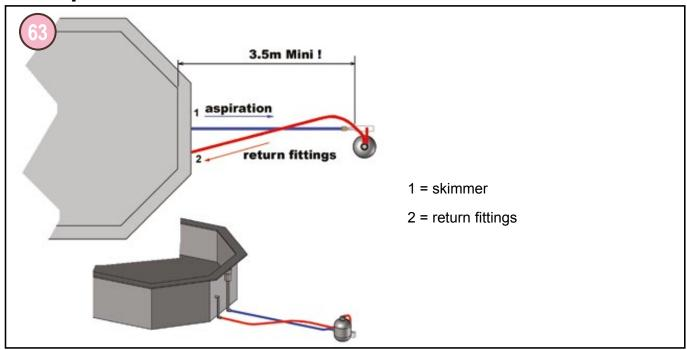
Connect the rigid descending pipes to the filtration group as shown above. The roll of tubing provided in the Filtration kit is sized for a standard installation, that is to say, with the filter group located 3.5 m from the pool (minimum distance between the pump and the pool according to the French electrical safety standard C15-100 if the filtration group is not installed in a locked plant room).
