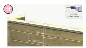
To hold the track in position, drive in a screw 2 cm from each end. Next finish attaching the track by driving in screws at 20 cm intervals. Use  $\emptyset4$  x 35 screws (bag D).
