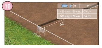
You will need to dig shallow trenches to hold the cradles. Make sure that these are parallel to each other and to the A2 axle. The number of trenches required will depend on the pool model, refer to the illustrations corresponding to your pool. Trenches should be regular and sized to hold the cradles in the right position.
