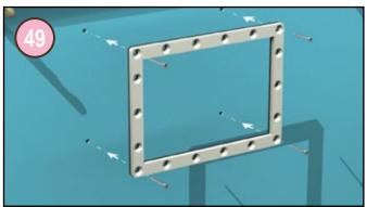
Glue the second skimmer gasket to the interior surface of the skimmer flange. (The interior surface has sharp edges while the exterior surface has rounded edge).
