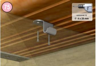
The wooden ladder is fitted with two lever latches that lock it into position. The lever sections are fitted to the ladder supports and the hooks are mounted under the coping (these parts are enclosed in bag K). Observe how these 2 parts interact together to understand how the mechanism works and establish the travel necessary for the ladder to be locked correctly into position.
