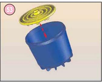
Place the collector plate in the base of the filter tank. Check that it is flat.
