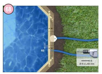
Screw the two side elements in position as shown...
