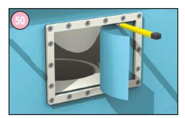
Cut away the liner inside the flange. Keep the offcuts for future repairs.
