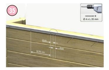
FixezHold the track in position using a screw placed 2 cm from each end. Then complete attachment of the track by inserting screws at 20 cm intervals. (Use Ø4 x 35 screws -sachet D).).
