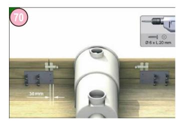
Study the illustration above. Mount the brackets (identical to the connecting brackets) as shown using screws (bag M).
