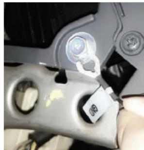
Connect the black GND terminal to a grounding source (e.g. metal component)
