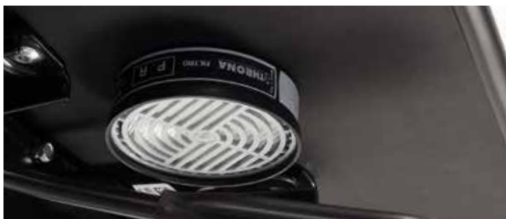
Detail of HEPA high filtration efficiency filter
