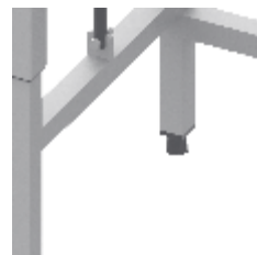
Welded frame. Legs made of stainless steel tube 40×40 mm. Frame made of stainless steel tube 25×25 mm
