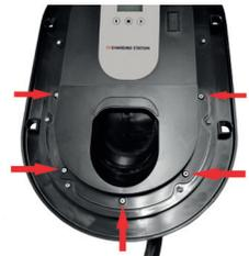
6. Use 4 wood screws M4,5x35mm to mount Charging Station on the wall. The Charging Station should be installed between 0,80m and 1,20m from bottom to the ground.
