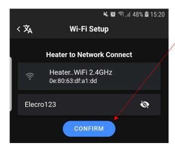
After approximately 30 seconds you should get confirmation on the phone that the connection was successful. If connected successfully the TS Controller will return to 'NORMAL'. If the connection failed then it will return to the 'CONNECT WiFi' option. Please try to connect again if this happens.
