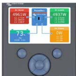
Color Control GX, showing a PV application
