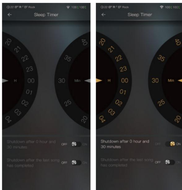
Set the count down sleep timer to power off the DX300. The left hand side is the value of hours. The right hand is the value of minutes. The DX300 will be powered off after the counter has completed. If there are any operations in the meanwhile, the DX300 will start the counter again after the last operation.
