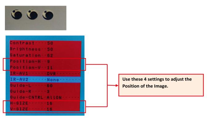
Engage Reverse Gear and fine position the image in same manner. User can also select if user wants to turn Guidelines ON or OFF and can also select if Parking Sensors are ON or OFF. For this again use the 3 buttons on the bottom of the interface to access the OSD menu. Once in the menu navigate to settings for "Guide-CNTRL" and select as desired.
