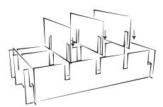
3. Slide the center uprights C into the horizontal plates A, as shown on the image. Put the closet upright and it's done!
