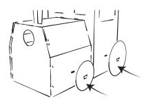
6. Click the back wheel F and front wheel G into the back and front of the train's side, respectively. Do the same on the other side.
