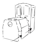
Fold B into the front part and fasten into the incisions of A. Close the front by clicking part C into B.
