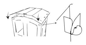
Connect the hooks in the top corners of body train A together as indicated on the image. Make sure these are folded inwards. Then fold roof D along the folding lines and fasten on top of part A.
