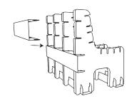
Slide the two large support beams D into the notches on the back of the legs.
