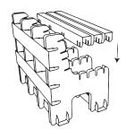
Slide the three beams B into the top notches of the legs.
