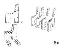
Take the eight legs A and slide them into the two support beams C, as shown in the image.
