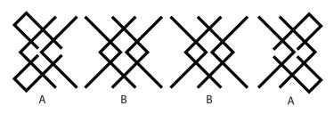
The frame consists of 4 parts. The front and rear parts (A) are the same, and are connected to the middle parts (B). See image for the overview.
