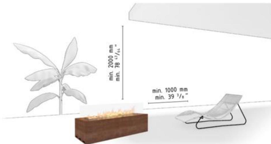
Figure 1: Minimum distance to flammable materials
