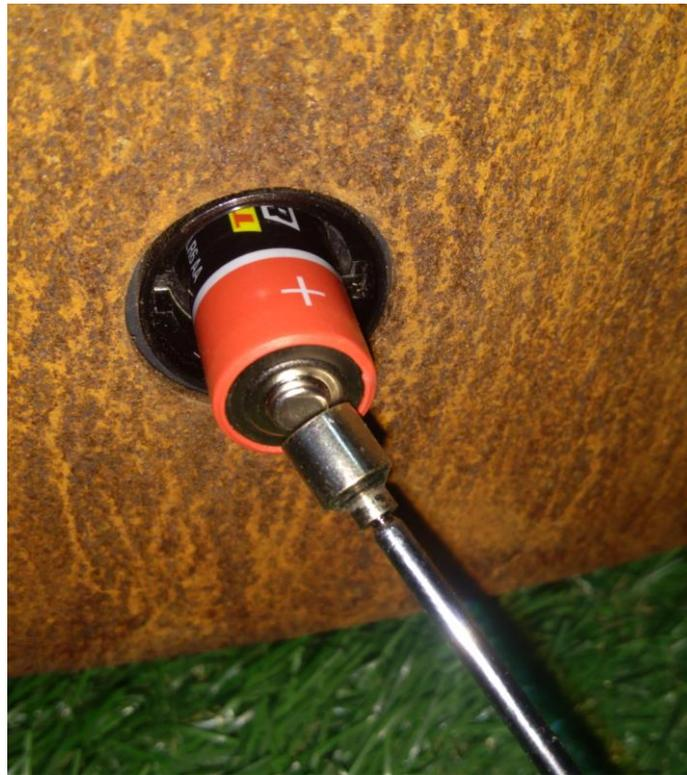
*Photo 8: Removing the first battery using the magnetic gripper*
