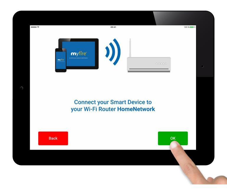
When the connection is established the myfire Wi-Fi Box leaves the Access Point Mode (Hot Spot) and is connected to your Wi-Fi Router.
