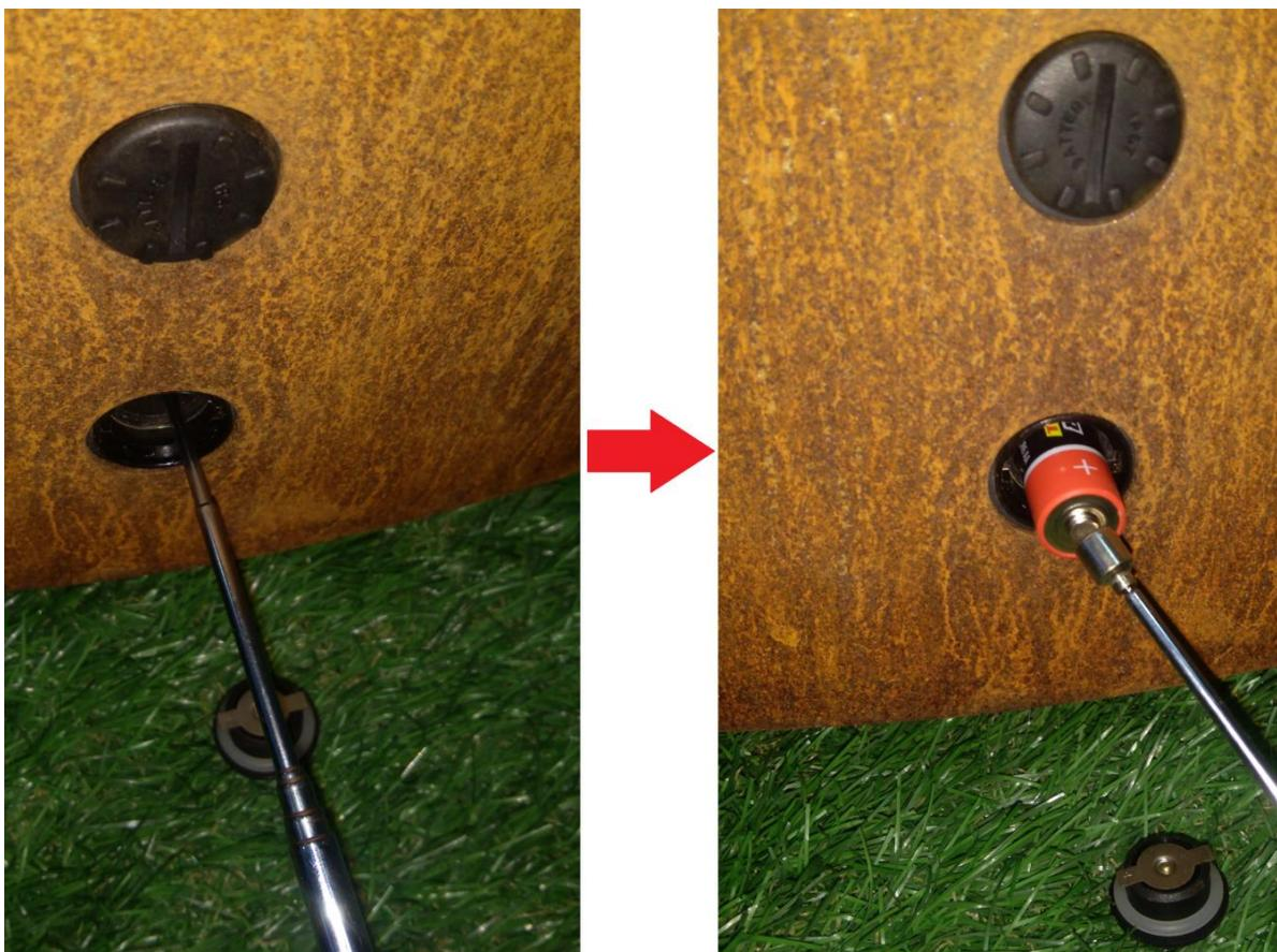
*Photo 8: Removing the second battery from the container*
