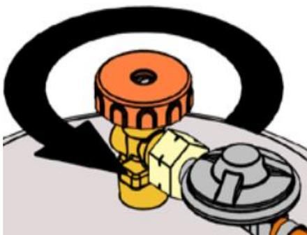
4. To let the gas flow in turn the switch into the ON position (or into the flame image).
