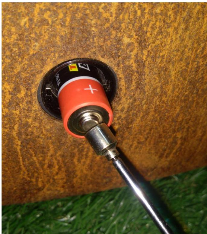
*Photo 7: Removing the first battery using the magnetic gripper*
