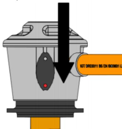
5. When the gas flow is required turn the valve of the bottle counter-clockwise.
