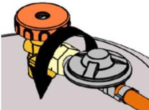
3. Place the quick-release regulator on the valve and press it down hard. If the switch is correctly turned off you will hear a characteristic click.
