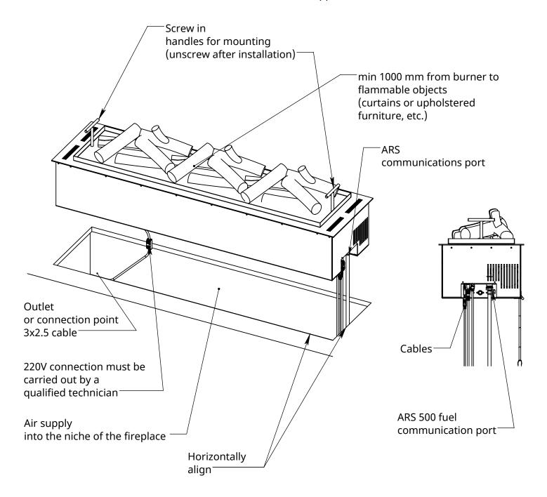
It is mandatory to use a separate line with a circuit breaker with a rating of at least 10A
