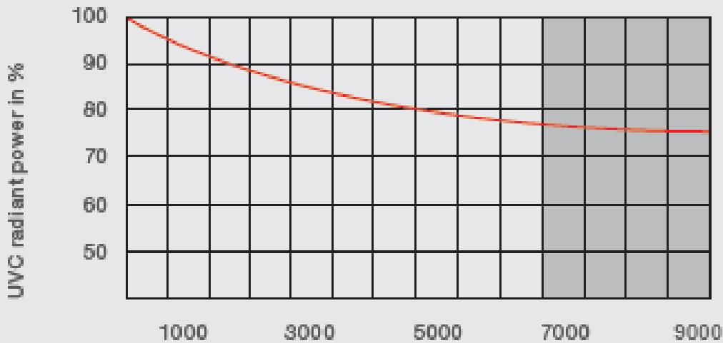
The lamps have a maximum life of 18,000 hours. To maximize the effectiveness of killing viruses and bacteria, we recommend replacing the lamps after 9,000 hours. The device signals the need to replace the lamp.
