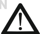
General warning: Warns the user about the presence of important operational and maintenance instructions in the documentation attached to the device.
