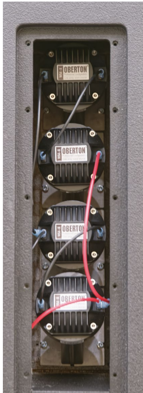
Tweeter unit of Venia-8 with four line array elements WS4, equipped with ND2545 drivers
