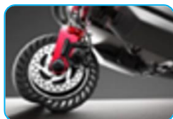
Shock-absorbing airless NPT tires
