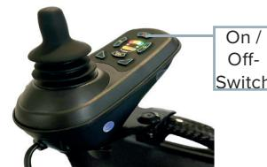
13. After use, switch off (remove the battery if not using for more than 48 hours). Then simply fold by releasing and holding away the folding clip, and push forward on the backrest. Stand the chair up right and store in a suitable location.
