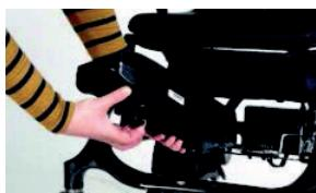
9. Install the seat cushion which attaches with Velcro.
