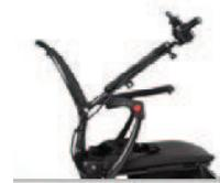
Install joystick by choosing preferred side, then turn the securement knob to loosen and then insert the joystick tubing. When the required position is reached, tighten the knob to secure. Connect the 2 terminals ensuring ends are locked in place.
