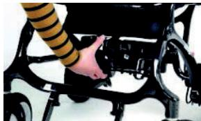
8. To insert battery. Slide the battery on to the rails underneath the seat. Push the battery firmly backwards until it locks in position with an audible click.
