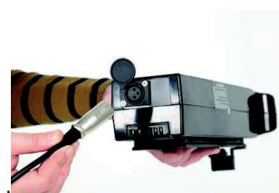
12. Ensure the charger is removed before operation and switch the powerchair on.
