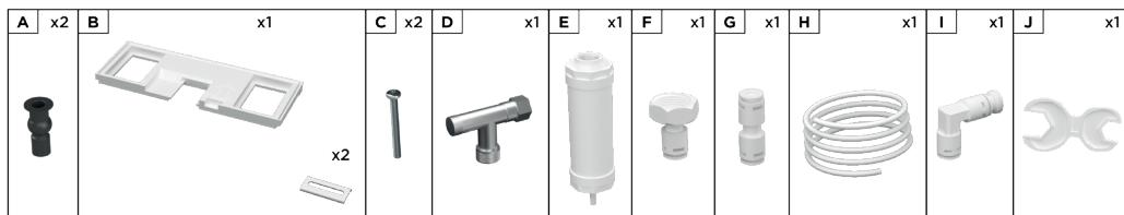
1 plate, 2 fixing hinges (extendable rubber nuts and screws), 2 perforated metal plates, 1 T-fitting, 1 angled quick coupling, 1 straight quick coupling, 1 threaded coupling, 1 plastic hose (1.15 m) and 1 filter.
