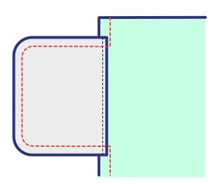
Continue stitching and close the side seam. Stop 1cm-3/8" after the notch for the slit.
