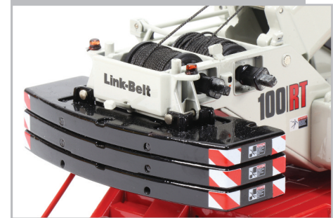
Above: There are two functional winches, both with a braking system.
