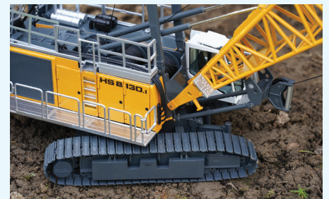
Additional undercarriage counterweight and fairlead for dragline operation.
