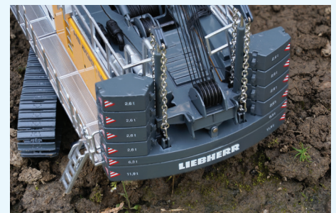
Counterweight with assembly cylinders and detailed printings.
