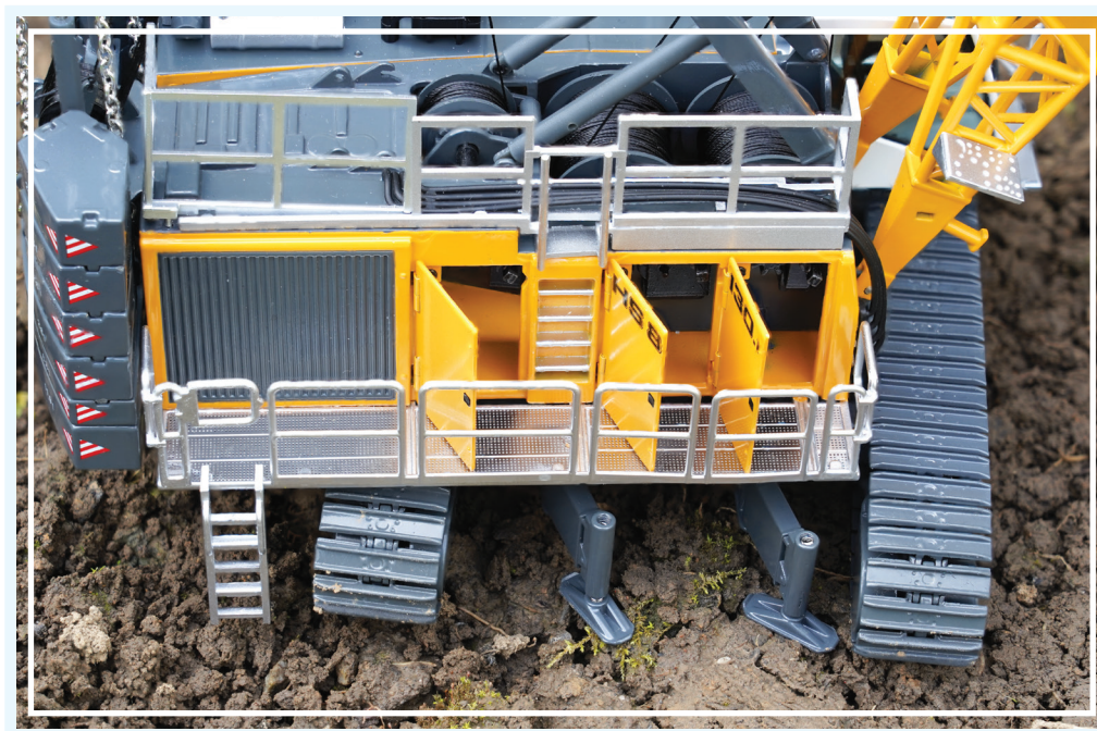
Doors with small hinges to hide winch operations.
