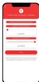
In the first screen you will be able to configure the maximum and minimum intensity between which the dynamic control will work. If your installation is limited to 20 amps, you will not be able to exceed the 20 amps indicated. Slide the drop-down to select the maximum intensity of your installation and the minimum intensity of your installation you want to charge.
