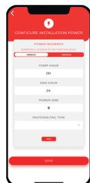
In the installation power configuration section, you will be able to select the maximum contracted power in the same one. Access it to configure the hourly time slots.
