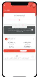
By accessing the recharging point configuration menu, it is possible to configure the recharging point via WIFI or Bluetooth (only devices with this configuration). The power configuration can only be done if the dynamic control is previously activated correctly.
