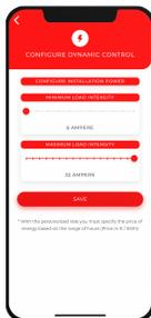
6. Specify the minimum recharge current (> 6 Amps) and maximum current (< 32 Amps). After select 'Configure installation power'.
