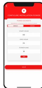
7. Establish different time slots and the maximum contracted power. In the case of having a single power range, add the timetable from 00:00 to 24:00 both daily and at weekends. If it is a photovoltaic installation, indicate the operating mode in each time slot (PV + Minimum power, Exclusive PV or Grid + Photovoltaic).
