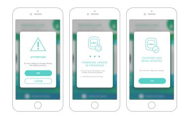
Note that the firmware update feature requires the charger to be connected to the Internet. At the end of the process, a confirmation message is shown.
