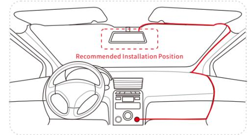
2)Rear car cam installation position & wiring method for power line
