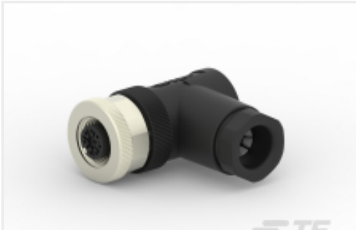
TE Part #T4112002081-000 M12,FEMALE,RA,A CODE,8P,PG9, GOLD
