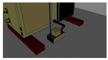
Drain pump of the condensation water
