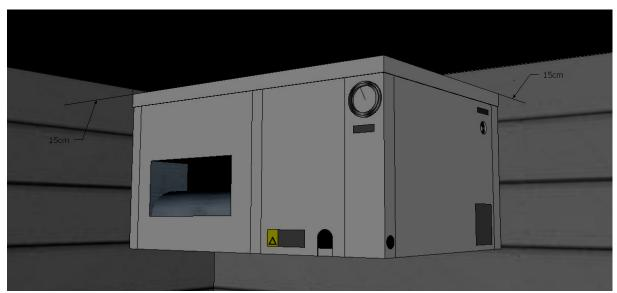
The unit should be mounted in such a way that the side of the condensation drain is at least 1 cm lower than the other side (slope) to ensure that the condensate drains properly. In practice, the 1 cm elevations at all corners – except the corner of the electrical compartment – are exactly right for a correct fall. Using a spirit level is recommended.
