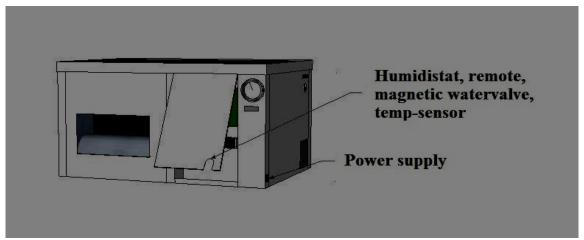
First, the panel at the left side near the manometer should be removed to make the various electrical connections.
