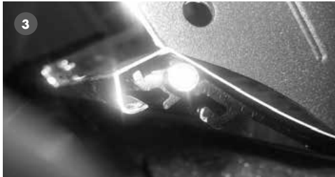
Pry end of reflector open
