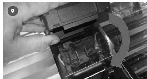
Slide fittings on both side of the lamp firmly towards the lamp
