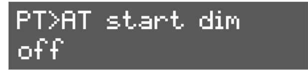
The crop does not vaporize adequately if the plant temperature is higher than the room temperature. The controller can intervene by dimming the lights and turning off the CO2 dosing. The difference in temperature can be set by pressing briefly on the SET key and using the + and – keys to fill in a value. A typical value is – for example, +2 degrees. The controller will intervene if the leaves of the crop are 2 degrees warmer than the room.
