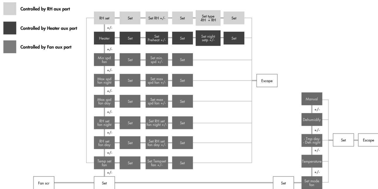
The two aux settings can be used to control the heating systems and the humidifiers and dehumidifiers. The menu structure is as follows:
