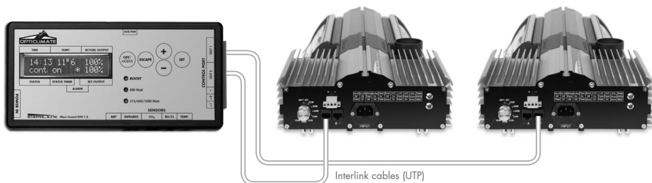
There are two ports on the ballasts or light fixtures, to which the Interlink cables are connected. The port on the Maxi Controller (out 1 and/ or out 2) is connected to port A of the ballast or light fixture. Port B is now connected to port A of the ballast or light fixture via an Interlink cable. The sequence is therefore controller-out> port A, then from B to A / B to A / B to A etc. A is therefore the input signal and B is the output signal.
