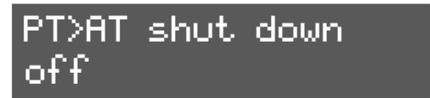
The plant temperature will increase further if the controller has intervened but no measures are taken to restart the vaporization. The controller will then shut down the lights completely if the plant temperature rises. The difference in temperature in which the controller shuts down all lights can be set in the PT>AT shut-down option. A typical value in which the controller does this is usually +2 degrees higher than in PT>AT Dim (therefore +4 degrees).
