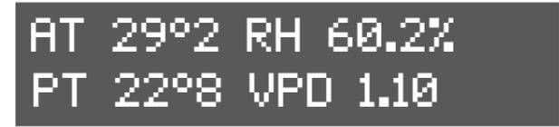
You can read the room temperature (AT), relative humidity (RH%), plant temperature (PT), delta-T (DT) and the VPD value on the VPD display screen. You can switch between PT and DT by pressing the + and – keys in this screen. PT is the plant temperature measured with the plant temperature camera. Delta-T indicates the difference between AT and PT.
