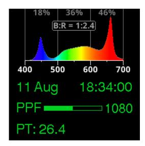
In the  $\square$  Manual program, both outputs can be adjusted independently or in conjunction, using four sliders in the menu. The  $\bigcirc$  Grow and  $\bigcirc$  Bloom programs greatly simply this by predefining the B:R ratio (not user configurable) and hiding the sliders in the menu, leaving only one control for the user. It's recommended to start with one of these  $(\bigcirc$  and move on to  $\square$  Manual once you are more familiar with the features and capabilities.
