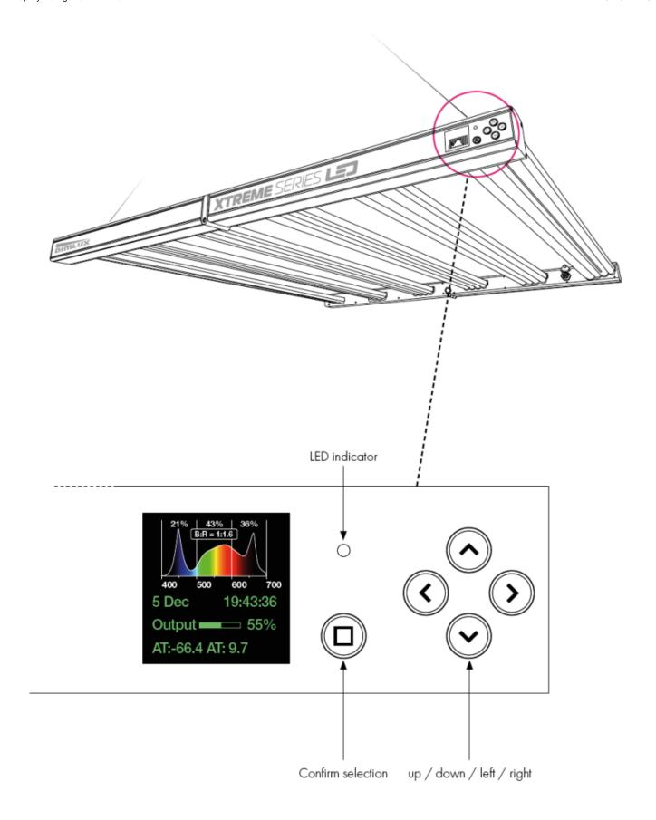
By pressing the button with the square you activate the display. Use the up/down arrows to navigate through the settings. If you are on a setting and use the right arrow you go to the subsettings / functionalities.
