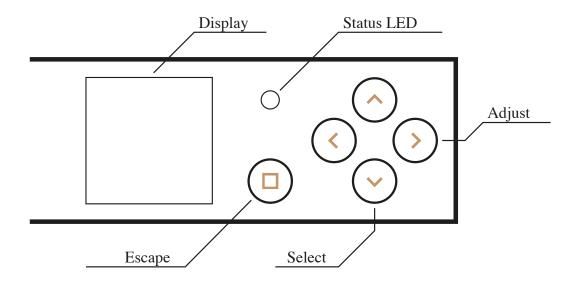
he display is a 1.54''  $240\times240px$  IPS panel. It shows a live color spectrum of the light output in the top half, and status, controls, and the menu in the lower half.
