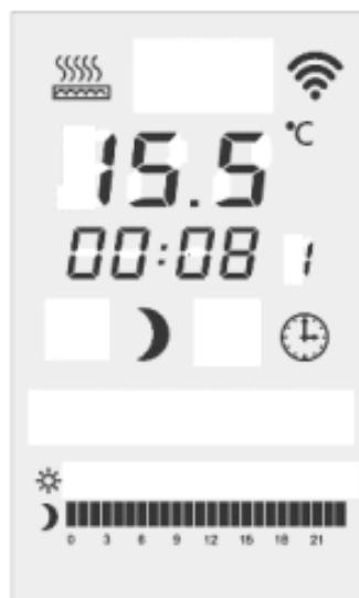
**Setting hours:** To set the hours, press and release the mode button (menu button). Then press ▲ or ▼ button to set the minutes within the range of 0–23 hours, in 1-hour increments. After 30 seconds without input, the setting will automatically end and the display will switch to the minute settings.
