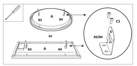
2. Secure the mounting template onto the ceiling, accurately identifying the corresponding hole positions, and mark the hole locations on the ceiling for drilling purposes. (Alternatively, you can determine the drilling positions by measuring the distances ab and ac on the back of the product.)
