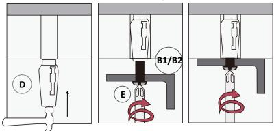
The expanding nut goes into the inside of the hole, it is strictly prohibited to install it in reverse!
