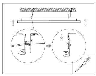
7. Secure the two brackets with screws(C2) and tighten the screws.
