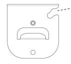
Insert the power cord into the Cable routing groove to lift it off the surface and ensure proper routing.
