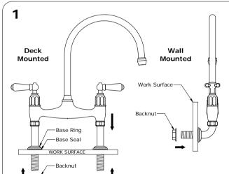
Ensure the mixer is orientated correctly, levers should rotate to point forward and hot index should be situated on the left.
