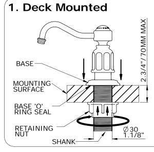
The diameter of the hole should be Ø30mm/1.1/8". The maximum thickness of the surface must not exceed 70mm/2.3/4"
