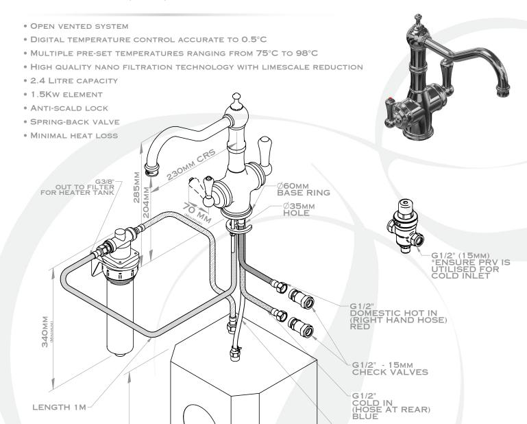
INLET TEMP RANGE: MIN 1°C / 34°F Max 85°C / 185°F
