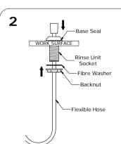
Secure rinse unit socket in a suitable position using a tap wrench or a 36 AF spanner.
