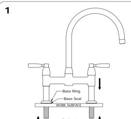
Ensure the mixer is orientated correctly, levers should rotate to point forward.
