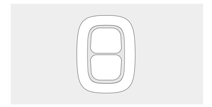
DoubleButton blinks red and green to indicate command execution and battery charge status.
