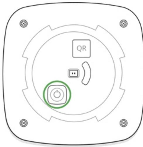
For the detection and interfacing to occur, the siren should be located within the coverage area of the wireless network of the hub (at a single protected object). If the device was already assigned to another hub, switch off HomeSiren and then perform the standard adding procedure.
