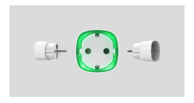
**Socket** is a wireless indoor smart plug with the power-consumption meter for indoor use. Designed as a European plug adapter (Schuko type F), Socket controls the power supply of electrical appliances with a load of up to 2.5 kW. Socket indicates the load level and is protected from overload. Connecting to the Ajax security system via a secured <u>Jeweller</u> radio protocol, the device supports communication at a distance of up to 1,000 m in line of sight.
