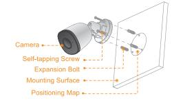
Step1 Drill screw holes on the mounting surface as the positioning map shows, and then put in the expansion bolts.
