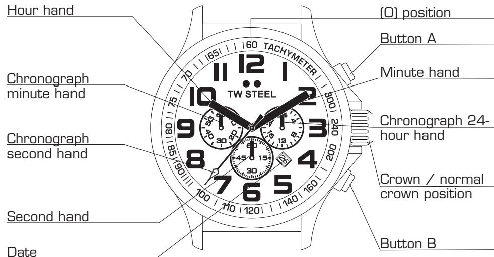
The chronograph hands can be advanced rapidly by continuously pressing button A. Once the chronograph second hand has returned to the (0) position, push the crown back to the normal position.
