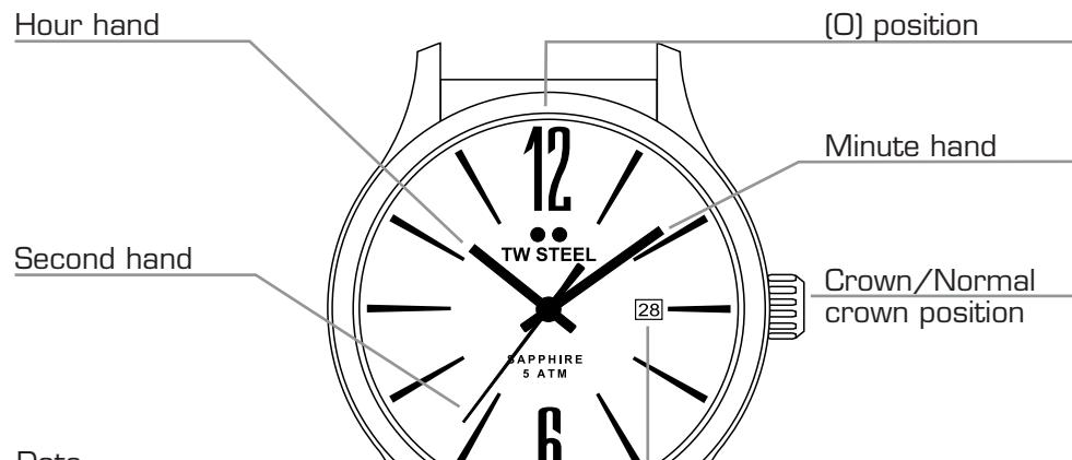
CAUTION : IF THE CROWN IS NOT PRESSED IN PROPERLY, THE WATCH IS NO LONGER WATERPROOF AND THE MOVEMENT CAN BE SERIOUSLY DAMAGED!
