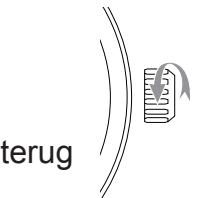
OPGELET: ALS DE KROON NIET GOED WORDT TERUGGEDUWD, IS HET HORLOGE NIET MEER WATERDIECHT EN KAN HET UURWERK ERNSTIG BESCHADIGD RAKEN!
