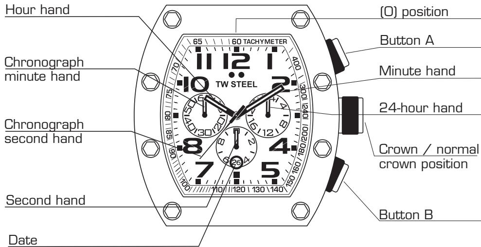
If the chronograph second hand and the chronograph 1/20 second hand do not return to the (0) position after the chronograph has been reset or after the battery has been replaced, you should do the following. Pull the crown out to the 2nd position. Press button A to set the chronograph second hand to the (0) position.
