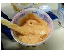
Transfer the complete LUWIREP 85 mixture into the second mixing cup!
